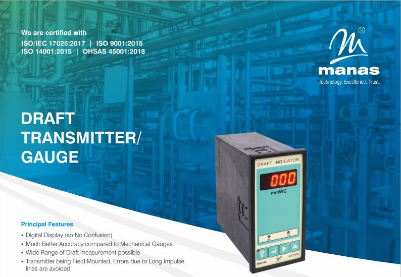
The Digital draft gauge 4475-PX accepts the draft pressure input as the signal and displays it in terms of mmwc. It also delivers 4 -20 mA output proportional to the Draft. The Draft transmitter is a field mounting unit and is a two wire system delivering 4 - 20mA output proportional to Draft Input.
